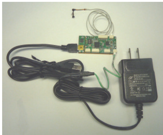
ST35B-14 Evaluation Kit connection
